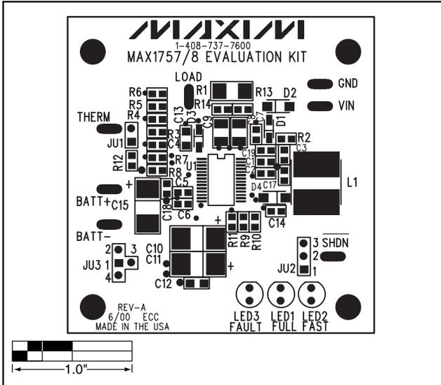
Figure 2. MAX1757/MAX1758 EV Kit Component Placement Guide—Component Side
