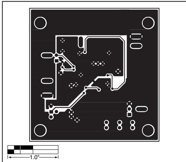
Figure 4. MAX1757/MAX1758 EV Kit PC Board Layout—Solder Side
