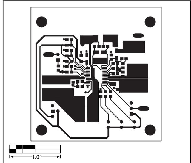
Figure 3. MAX1757/MAX1758 EV Kit PC Board Layout—Component Side
