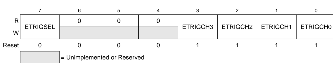
Figure 7-4. ATD Control Register 1 (ATDCTL1)
