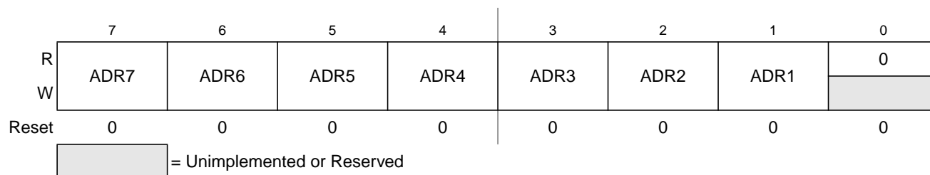
Figure 11-2. IIC Bus Address Register (IBAD)
