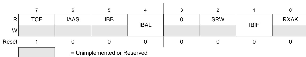
Figure 11-6. IIC Bus Status Register (IBSR)
