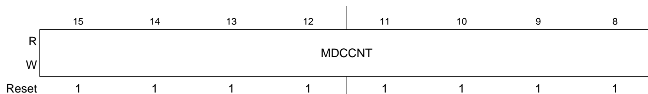
Figure 10-6. Modulus Down-Counter Count Register High (MDCCNT)
