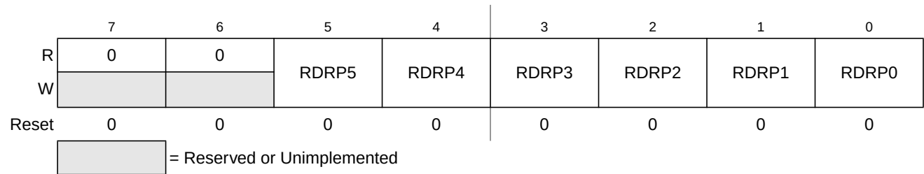
Figure 4-26. Port P Reduced Drive Register (RDRP)
