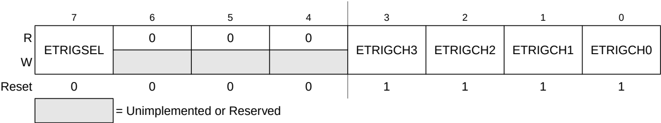
Figure 7-4. ATD Control Register 1 (ATDCTL1)
