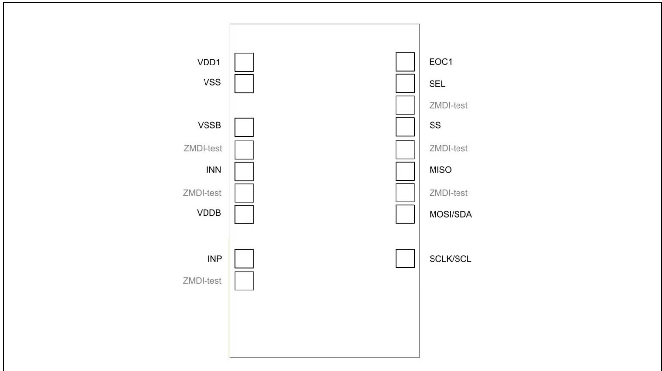
Figure 4.1 ZSSC3036 Pad Assignments
