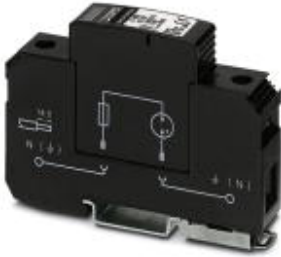
Surge arrester type 2, consisting of base element and protective plug with N-PE total current spark gap for mounting on NS 35/7.5, housing width: 17.5 mm (1 Div.)
