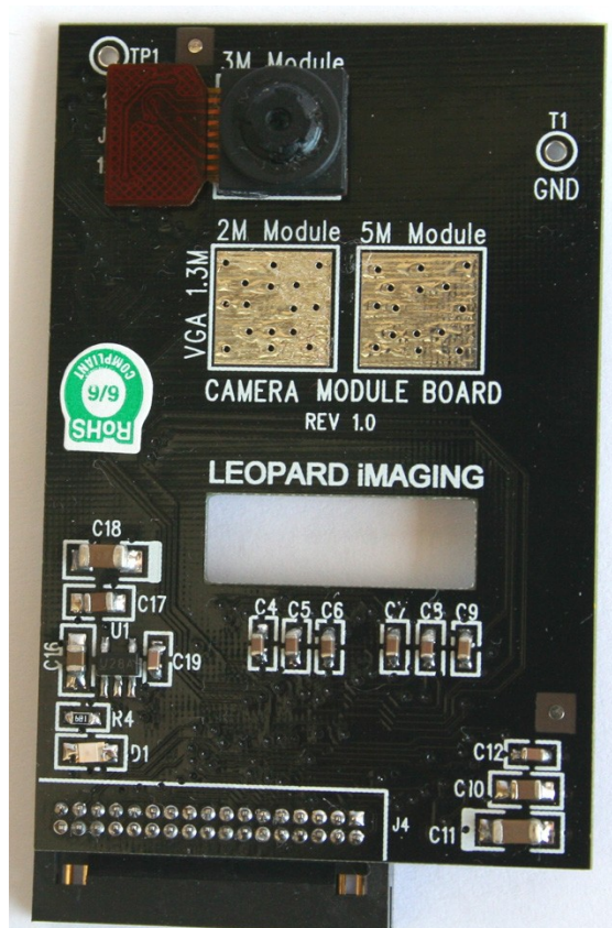
Figure 10. 3M Camera Board
