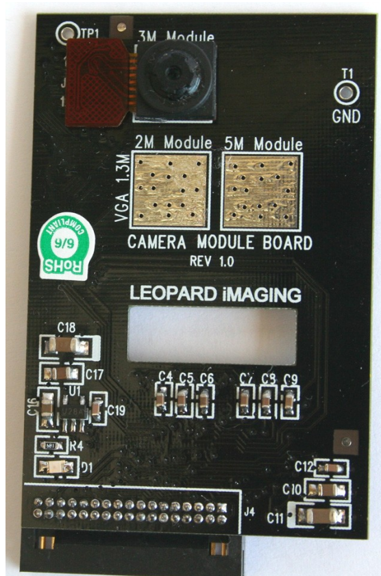
Figure 10. 3M Camera Board
