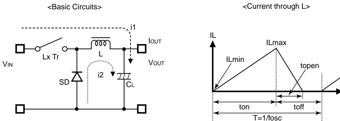
Step 1 :LxTr turns on and current IL ( $=i_1$ ) flows, and energy is charged into CL. At this moment, IL increases from ILmin ( $=0$ ) to reach ILmax in proportion to the on-time period (ton) of LxTr.
