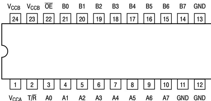
Figure 1. 24-Lead Pinout
