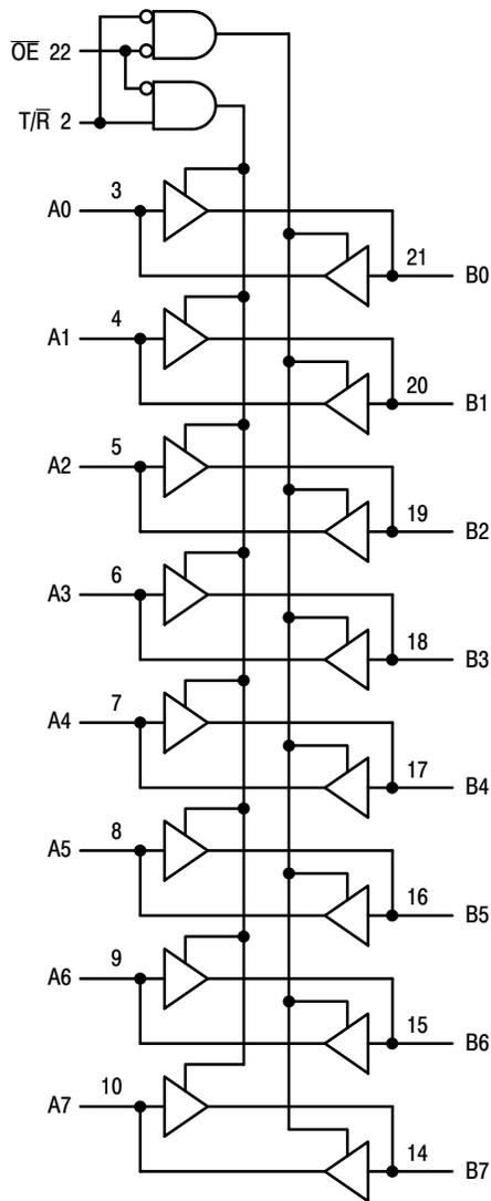
Figure 2. Logic Diagram
