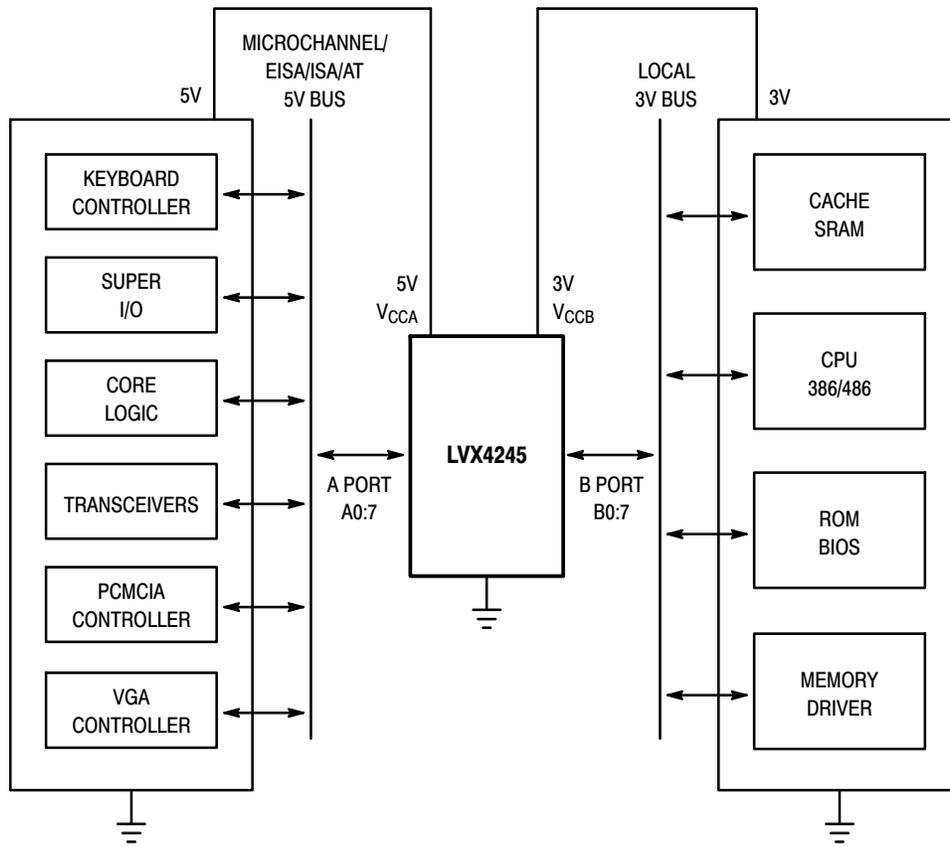
Figure 4. MC74LVX4245 Fits Into a System with 3V Subsystem and 5V Subsystem
