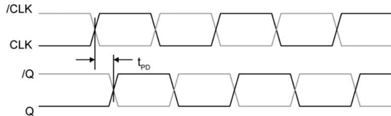
$t_{PD}$  – Differential In-to-Differential Out
