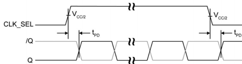
$t_{PD}$  – CLK\_SEL-to-Differential Out
