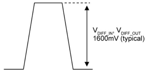
Figure 1b. Differential Voltage Swing
