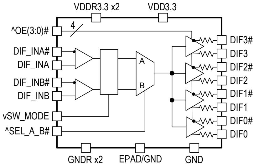
**Note:** Resistors default to internal on xx41/xx51 devices. P1 devices have programmable default impedances on an output-by-output basis.
