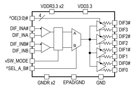
Note: Resistors default to internal on xx41/xx51 devices. P1 devices have programmable default impedances on an output-by-output basis.
