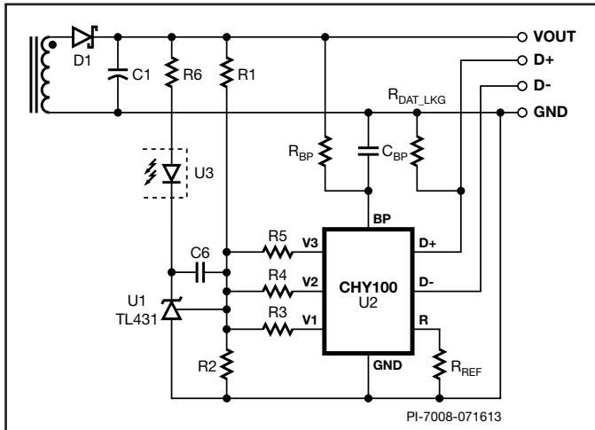
Figure 5. CHY100 with Traditional Output Regulation (CV Only).
