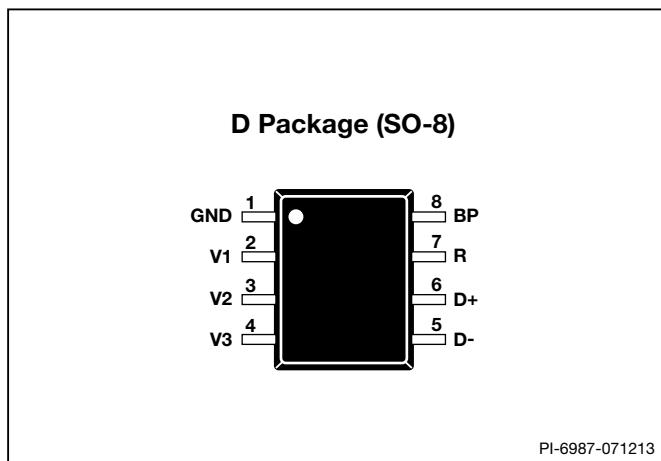
Figure 4. Pin Configuration.
