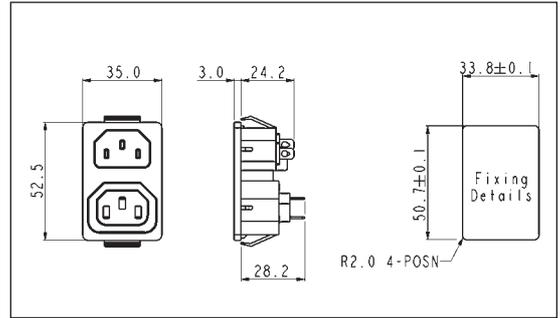
**SNAP FIT TO PANEL FUSED INLET/OUTLET**
