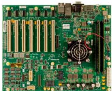
The dual memory controllers of the P5040DS support 4 GB of DDR3 at 1600 MHz. It has 128 MB of NOR flash, 1 GB NAND flash, a 256 KB IC EEPROM and two SPI memories: 16 MB flash and 128 KB EEPROM. It also has two USB 2.0 receptacles and an SD card slot.
