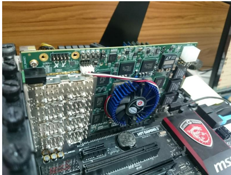
Figure 7-9 FPGA board installation on PC
