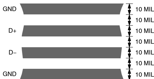
Figure 18. Typical Arrangement of Signal Tracks
