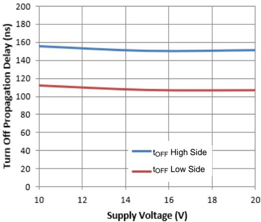
**Figure 6.** Turn-off Propagation Delay vs. Supply Voltage
