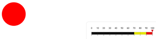
Figure 6-78. LED and slider control output at close proximity to sensor
