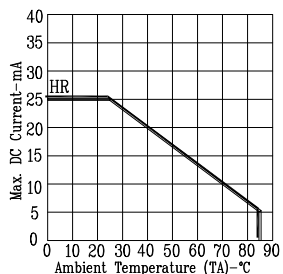
Fig5. MAX ALLOWABLE DC CURRENT VS. AMBIENT TEMPERATURE.
