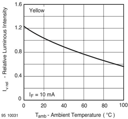
Figure 11. Rel. Luminous Intensity vs. Ambient Temperature
