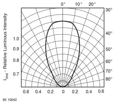
Figure 4. Rel. Luminous Intensity vs. Angular Displacement
