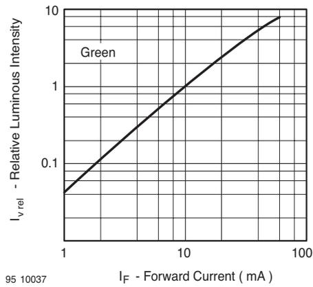
Figure 18. Relative Luminous Intensity vs. Forward Current
