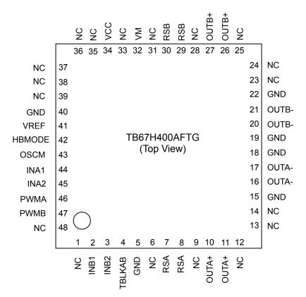
Note: Please connect the WQFN package corner pad and the exposed pad to the PCB ground pattern.
