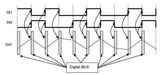
The Digital tBLK is inserted at the beginning of each charge period of the constant current chopping, and also when either of INA1, INA2, INB1, or INB2 is switched.
