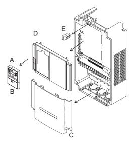
$oldsymbol{2}$  Cut out the two plastic break-outs from the front cover.
