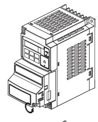
2 Pull the DeviceNet Communications Unit straight out of the inverter while pushing down on the indicated sides to release the snap-fits.
