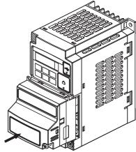
6 Press down on the indicated corner of the **DeviceNet Communications Unit housing to ensure** proper connection of the DeviceNet Communications Unit connector.
