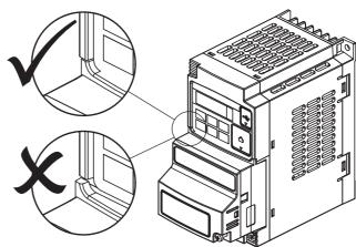
8 Secure the DeviceNet Communications Unit in place to the inverter with the mounting screw.
