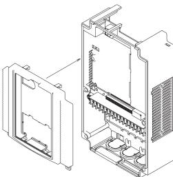
**4** Connect the connector of inverter connection PCB of DeviceNet Communications Unit to the connector of inverter.
