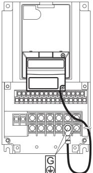
**9** Reinstall the terminal cover and tighten the two screws to fix it in position.
