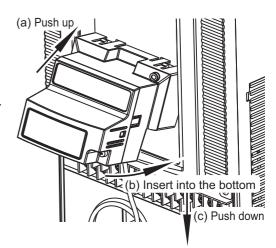
7 Insert the DeviceNet Communications Unit fixation screw into the hole shown in the right figure, and tighten it to fix the Unit.
