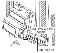
Remove the Inverter connection PCB by holding at the indicated locations.
