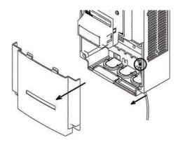
3 Remove the grounding cable of inverter.
