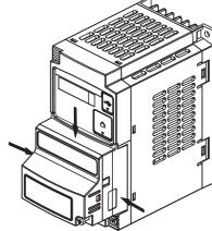
**3** For Inverters up to 4.0 kW, loosen the screws of the terminal block cover to remove the cover.
