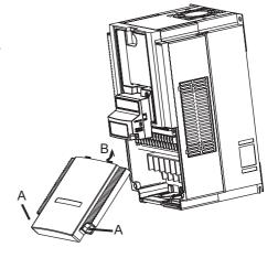
10 Install the Digital Operator above the DeviceNet Communications Unit.
