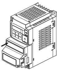
7 Check that there is no gap between the top edges of the DeviceNet **Communications Unit and the** inverter casing.
