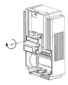
8 Connect the grounding cable of the DeviceNet Communications Unit to the ground terminal of the inverter.
