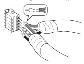
Use a dedicated crimp terminal to crimp the two wires inserted into the same hole, as shown below.
