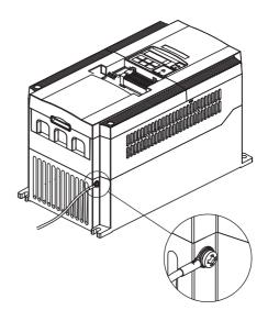
4 If removed in Step 2, reinstall the terminal cover and tighten the screw.
