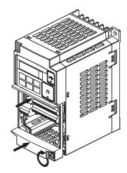
**5** Push the DeviceNet Communications Unit into the previous location of the DeviceNet Communications Unit cover until it clicks into place.
