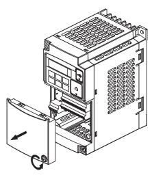
**2** For Inverters up to 4.0 kW only: Loosen the screws of the terminal block cover.
