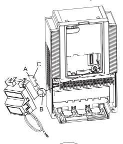
Then, align the larger hole on the Inverter connection PCB (C) with the threaded hole (F) in the Inverter. Push the Inverter connector into place.
