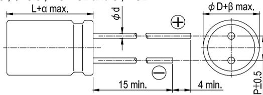
Lead Spacing and Diameter Unit: mm
