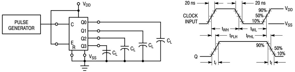
Figure 2. Switching Time Test Circuit and Waveforms
