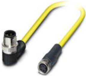
Sensor/Actuator cable, 4-position, PVC, Yellow RAL 1021, Plug angled M12-SPEEDCON, A-coded, on Socket straight M8, Cable length: 1.5 m
