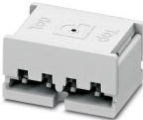
Plug component, Nominal current: 10 A, Rated voltage (III/2): 24 V, Number of positions: 4, Pitch: 2.4 mm, Color: white, Contact surface: Tin, for flexible PCBs with a width of 10 mm and a permissible PCB thickness in the contact zone of 0.15 mm ... 0.3 mm
