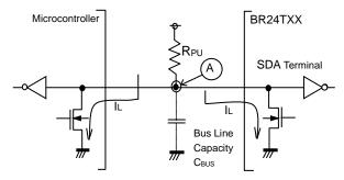
Figure 44. I/O Circuit Diagram
