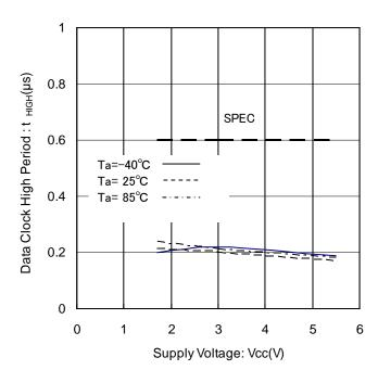
Figure 14. Data Clock High Period vs Supply Voltage
