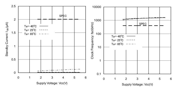
Figure 12. Standby Current vs Supply Voltage
