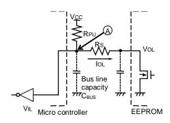
Figure 47. I/O Circuit Diagram
