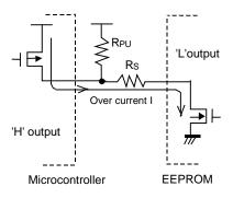
Figure 48. I/O Circuit Diagram
