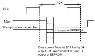
Figure 45. I/O Circuit Diagram
