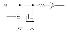
Figure 50. Input / Output Pin Circuit Diagram
