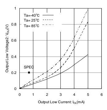
Figure 7. Output Low Voltage2 vs Output Low Current (Vcc=1.6V)
