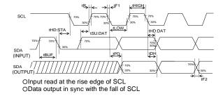
Figure 2-(a). Serial Input / Output Timing
