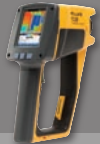
Fluke Ti20 Thermal Imager
