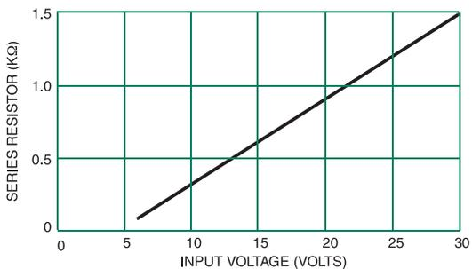
SERIES LIMIT RESISTOR VS INPUT VOLTAGE
