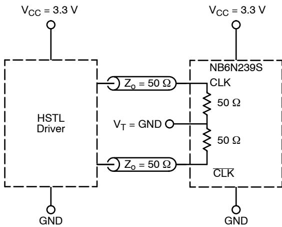
**Figure 15. Standard 50 Ω Load HSTL Interface**
