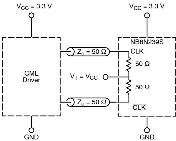
**Figure 14. Standard 50 Ω Load CML Interface**
