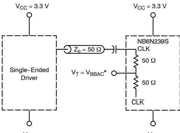
**Figure 17. Capacitor-Coupled Single-Ended Interface (V<sub>T</sub> Connected to V<sub>BBAC</sub>)**
