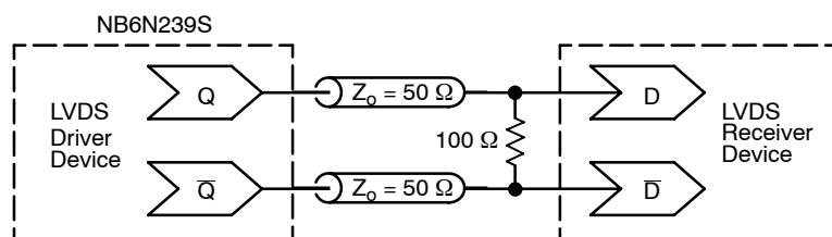
**Figure 20. Typical LVDS Termination for Output Driver and Device Evaluation,
