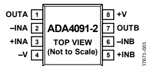
Figure 1. 8-Lead, Narrow-Body SOIC (R-8)
