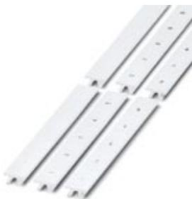
Zack marker strip, Strip, white, Unlabeled, Can be labeled with: Plotter, Mounting type: Snap into tall marker groove, For terminal block width: 15.2 mm, Lettering field: 10.5 x 15.1 mm
