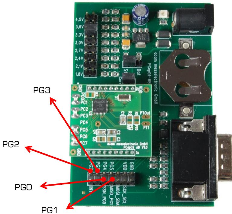
Figure 2-4: General purpose interface ports PGO to PG3
