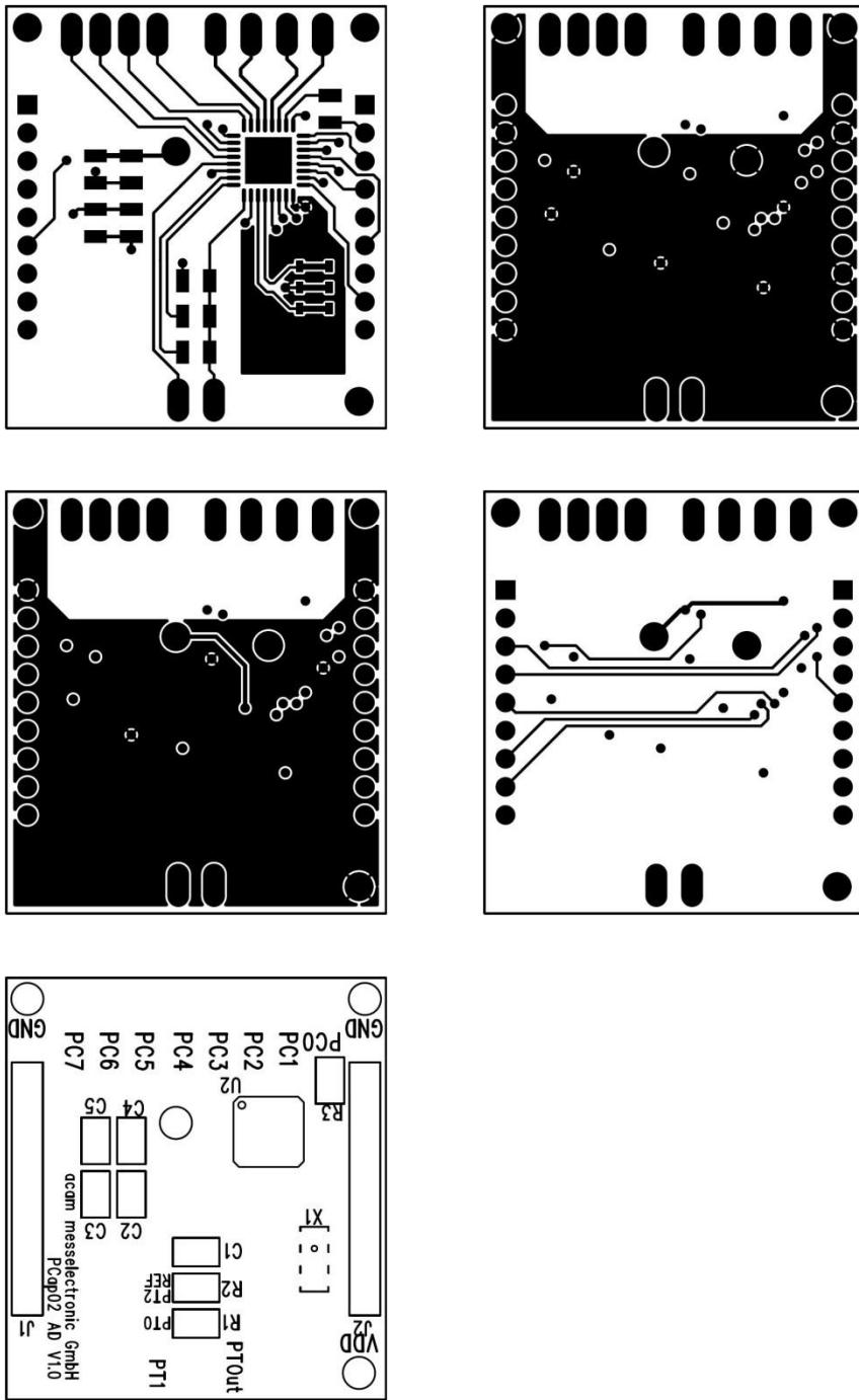
Figure 4-3: PCap02 AD module layout
