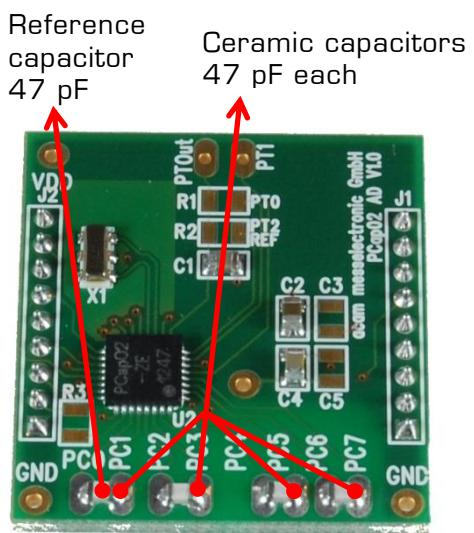
Figure 2-2: Details of the plug-in module
