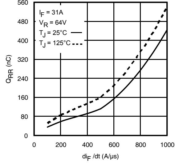
Fig. 19 - Typical Stored Charge vs.  $di/dt$
