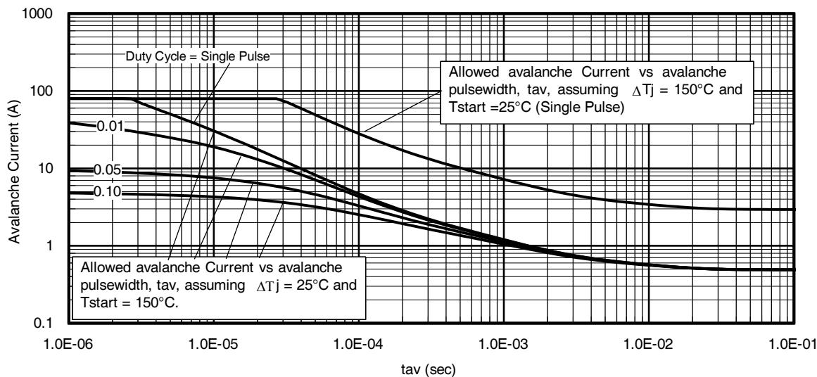
Fig 14. Typical Avalanche Current Vs. Pulse width
