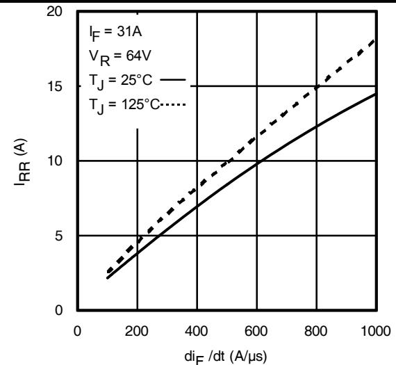
Fig. 17 - Typical Recovery Current vs.  $di/dt$
