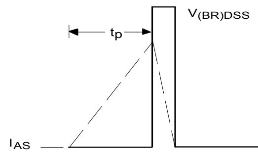
**Fig 21b.** Unclamped Inductive Waveforms
