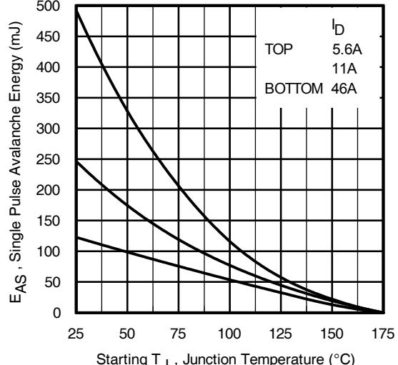
**Fig 12.** Maximum Avalanche Energy vs. Drain Current
