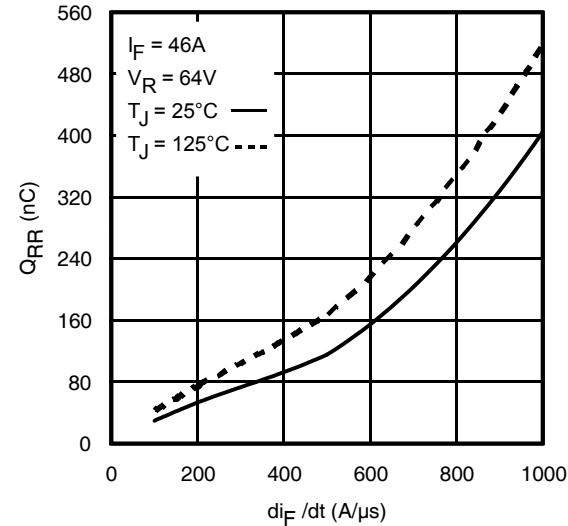
Fig. 20 - Typical Stored Charge vs.  $di/dt$
