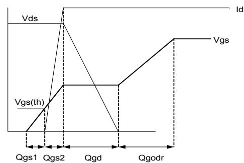
**Fig 23b.** Gate Charge Waveform
