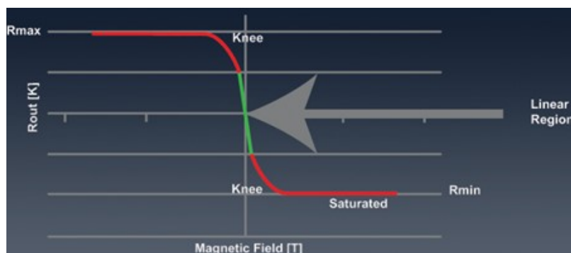
Figure 2: MTJ Response to a Magnetic Field
