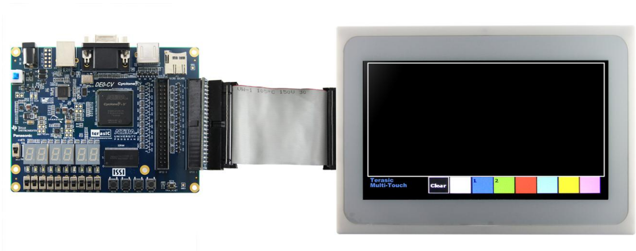
Figure 5-7 Hardware Setup with DE0-CV
