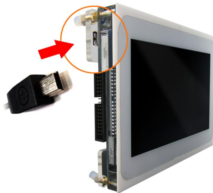
Figure 1-3 External USB Power Connection Setup
