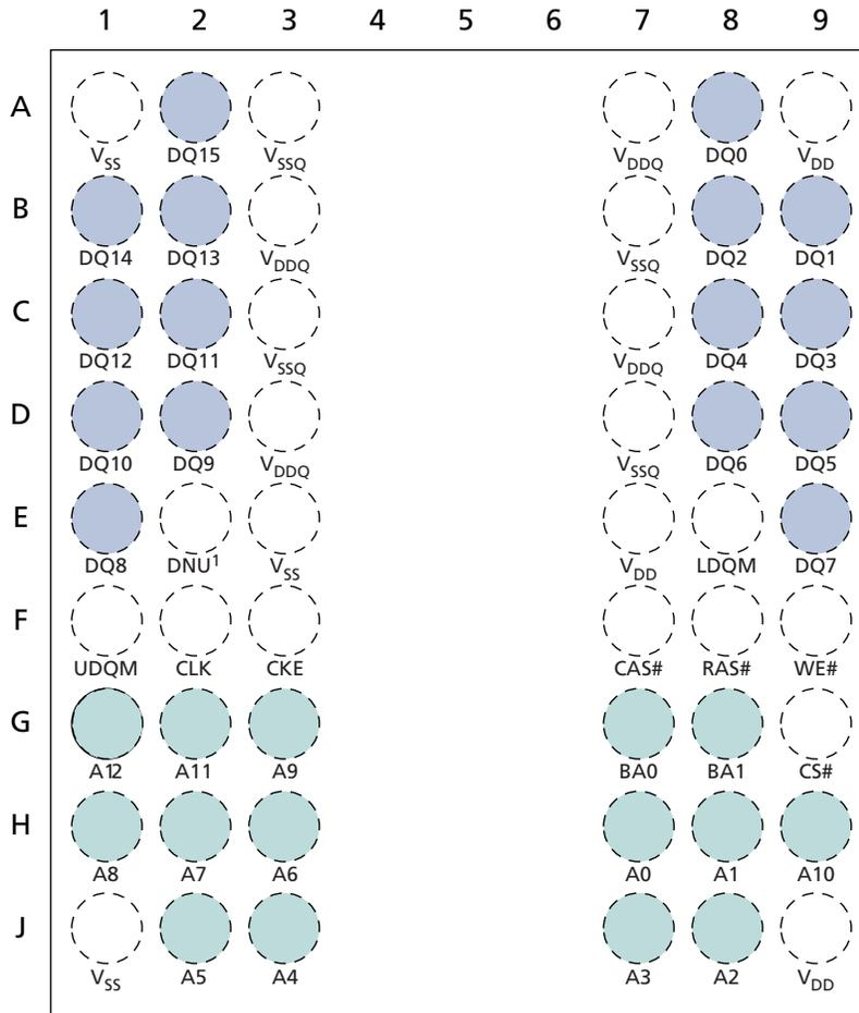
Note: 1. The E2 pin must be connected to V<sub>SS</sub>, V<sub>SSQ</sub>, or left floating.
