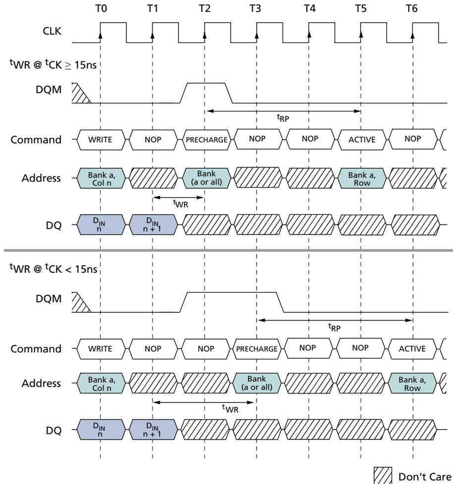
Note: 1. In this example DQM could remain LOW if the WRITE burst is a fixed length of two.
