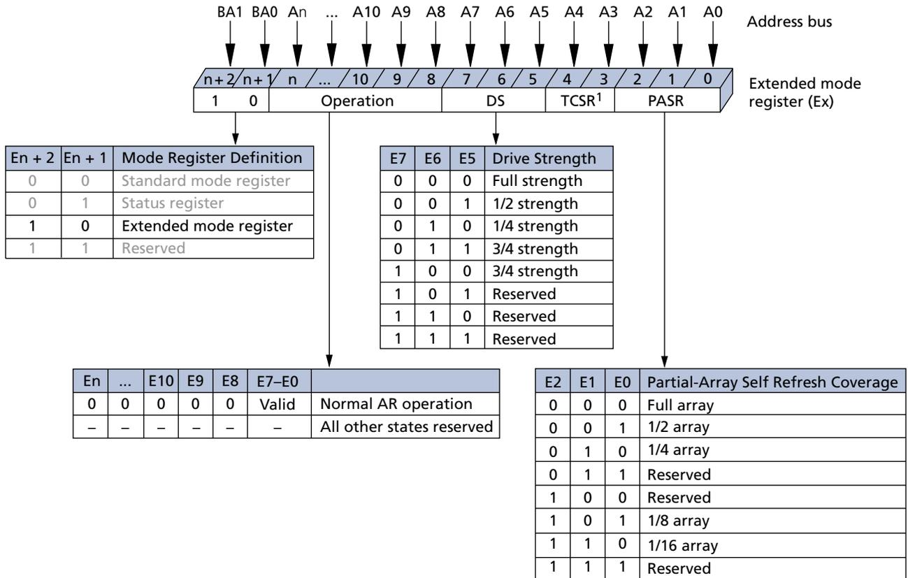
Note: 1. On-die temperature sensor is used in place of TCSR. Setting these bits will have no effect.
