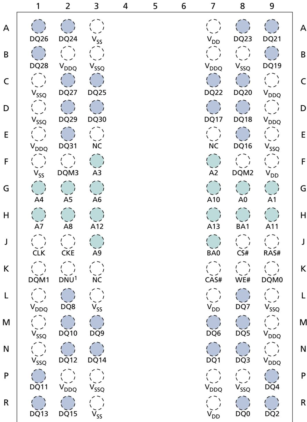
Note: 1. The K2 pin must be connected to V<sub>SS</sub>, V<sub>SSQ</sub>, or left floating.
