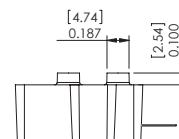
C- Two Ports Cut 0.100" Configuration
