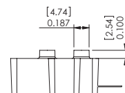
C- Two Ports Cut 0.100" Configuration
