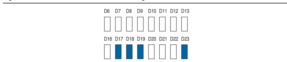
Figure 4-11. Condition of LEDs for Transmitting SDI-SDI Video Standard
