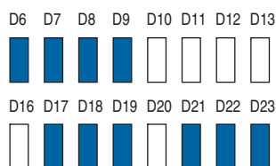
Figure 4-13. Condition of LEDs for Transmitting 3G-SDI Level A Video Standard
