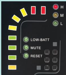
Extech's Refrigerant Leak Detector is easy to use and is ideal for detecting leakages from air-conditioning units and cooling systems that use all standard refrigerants. The multi-colored LED light bar indicates the level of leaking refrigerant detected by the RD300. The built-in, bright LED convenience light located at the sensor tip illuminates dimly lit inspection areas.
