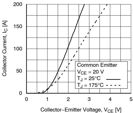
**Figure 4. Typical Saturation Voltage
