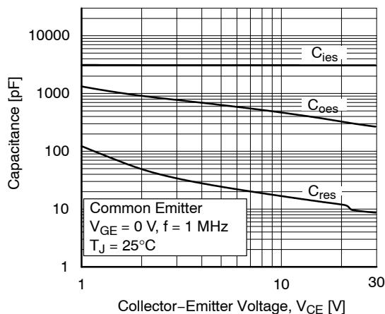
**Figure 8. Capacitance Characteristics**
