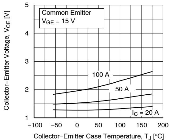
**Figure 5. Saturation Voltage vs. Case Temperature
