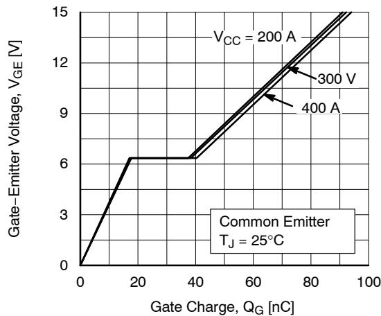
**Figure 9. Gate Charge Characteristics ( $T_J = 25^\circ\text{C}$ )**
