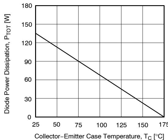
Figure 19. (Diode) Power Derating
