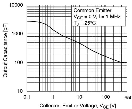
Figure 20. (Diode) Output Capacitance (Coes) vs. Reverse Voltage
