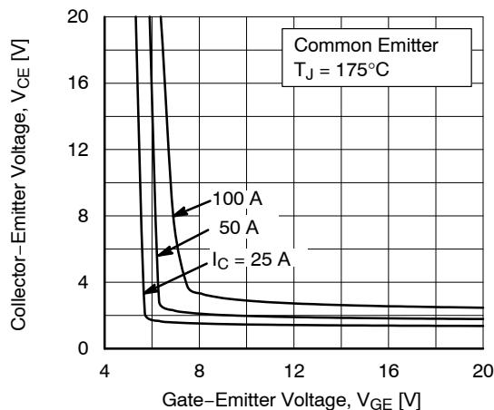
**Figure 7. Saturation Voltage vs.  $V_{GE}$  ( $T_J = 175^\circ\text{C}$ )**
