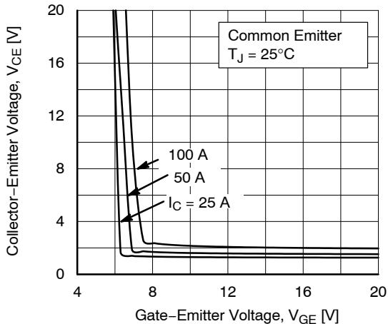
**Figure 6. Saturation Voltage vs.  $V_{GE}$  ( $T_J = 25^\circ\text{C}$ )**
