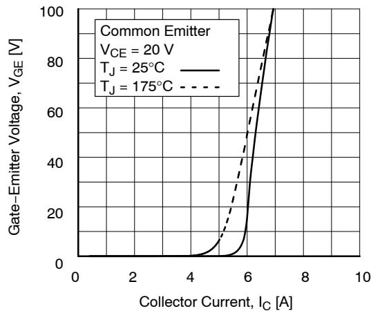
**Figure 3. Transfer Characteristics**
