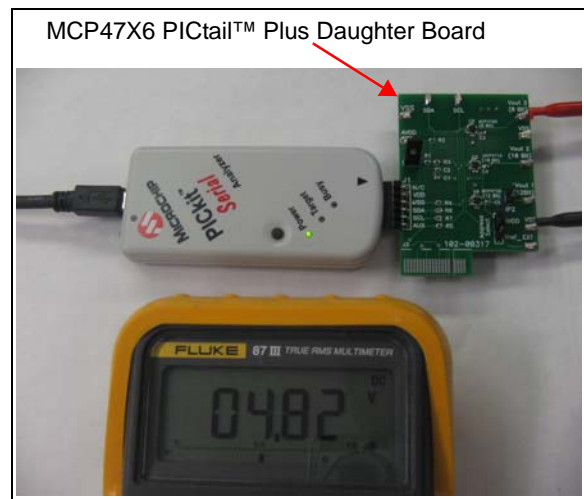
FIGURE 9-2: MCP47X6 PICtail™ Plus Daughter Board with PICKit™ Serial Analyzer.
