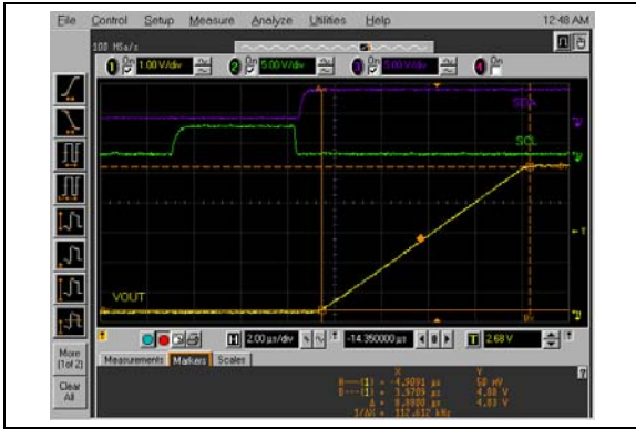
FIGURE 2-96: Full-Scale Settling Time (000h to FFFh) (MCP4726).
