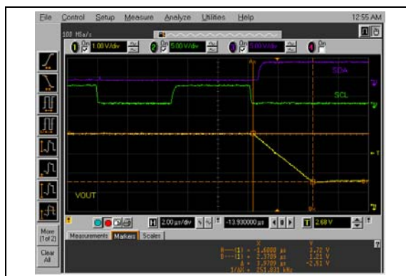
FIGURE 2-99: Half-Scale Settling Time (C00h to 400h) (MCP4726).
