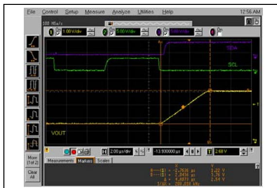
FIGURE 2-98: Half-Scale Settling Time (400h to C00h) (MCP4726).
