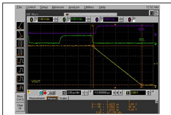
FIGURE 2-97: Full-Scale Settling Time (FFFh to 000h) (MCP4726).
