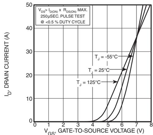
Figure 4, Transfer Characteristics
