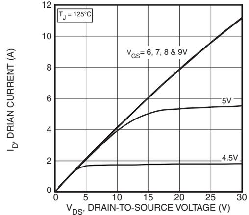
Figure 2, Output Characteristics
