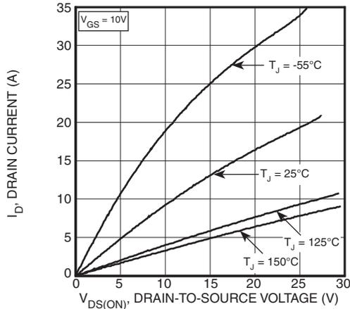
Figure 1, Output Characteristics
