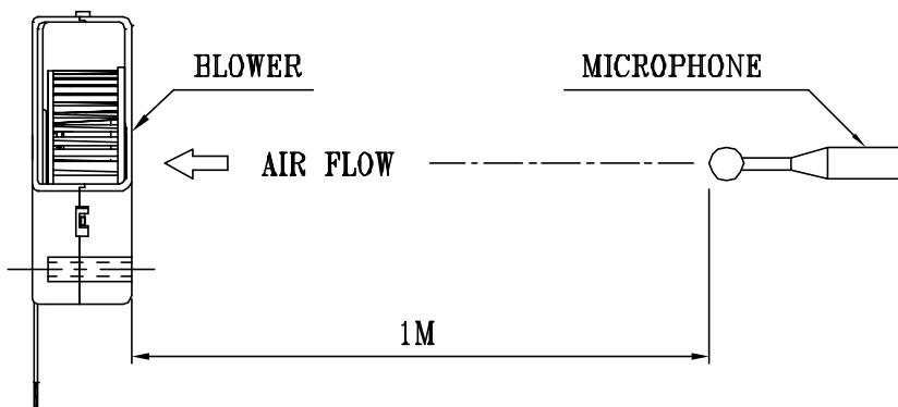
NOISE IS MEASURED AT RATED VOLTAGE IN FREE AIR IN ANECHOIC
