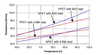
Output resistance were measured under the condition of V<sub>CC</sub> = 5.0V, V<sub>OPT</sub> = 5.0V, and V<sub>EE</sub> = -5.0V, with load resistors from outputs to ground.
